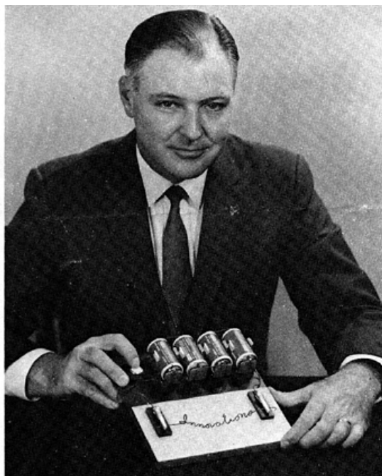
FIGURE 1. WILLIAM J. BUEHLER IN 1968, PICTURED WITH A DEMONSTRATION OF NITINOL WIRE. ELECTRICITY WAS PASSED THROUGH A STRAIGHT PIECE OF WIRE, AND THE WIRE WOULD CHANGE INTO THE WORD “INNOVATIONS.” THE OAK LEAF, U.S. NAVAL ORDNANCE LABORATORY, WHITE OAK, MARYLAND, JUNE 1968.
